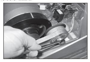
b. Lift up on the Tension Wheel and slide the motor drive belt over pulley to remove.
