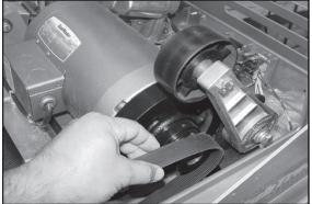
2.3 Use a 13-millimeter open-end or socket wrench to remove the four (4) hex nuts securing the motor to the headframe, and pull the motor off of the headframe.
